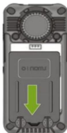
When installing the battery, insert the teeth at the top of the battery into the corresponding notches of the mobile phone, then press the battery down and secure it by turning the two screws. Ensure that the battery is safely installed before powering on the phone.
