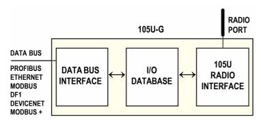
The 105U radio protocol is designed for very efficient radio usage, with configurable communications based on event reporting (I/O change), update times and/or poll response. Other features are:
