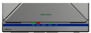
The following table is a summary for the wireless settings and LED displays. You can check the status of the AWK-4121 by reading these LEDs. More information about "Basic Wireless Settings" is presented in Chapter 3.
