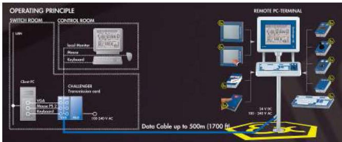
The CHALLENGER Remote PC Terminals represents the modern form of local operation in the production plant. All components for operation and visualisation are made intrinsically safe and certified world-wide. In this way configuration according to the specific conditions of the production plant is made possible. The configuration listed here is the standard - further configurations can be found under <http://www.gecma.com/configurator>
