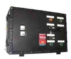
The JCE range of Power Inverter Units are intended for use in areas made potentially hazardous by the presence of flammable liquids, gases or vapours (Zone 1 and Zone 2). Certified for Group IIB and H<sub>2</sub> locations.
