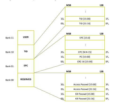
The inventory process returns the EPC code that is part of the content of the EPC memory bank as a side-effect of the singulation process. All the memory content, anyway, can be read using the Gen2 Read command and the rewritable memory can be written using the Gen2 Write command.
