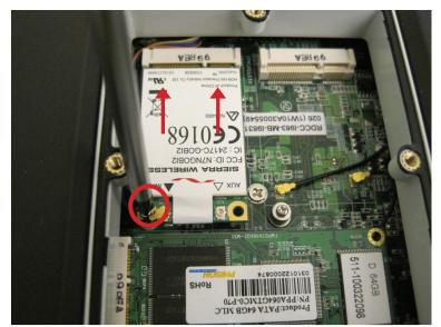
f) Place the WLAN card back to its original position by inserting it in its connector and gently hold down the card while you attach the silver screw.
