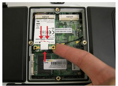
b) Unscrew the small silver screw in the lower left corner on the WLAN card.
