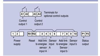
Outputs Isolated single pole, voltage free solid state
