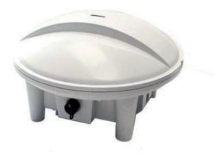
Zebra Location Solutions offers a heavy duty version of the WherePort III Tag Exciter that is designed for mobile outdoor environments. The WherePort III HD Tag Exciter is used to indicate proximity between mobile devices in harsh environments. It is capable of withstanding higher levels of shock and vibration than the standard WherePort III. It is sealed against dust and water, and it has been designed to be utilized in rugged outdoor applications.
