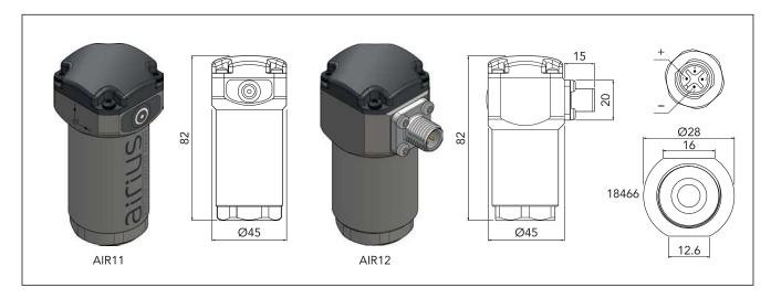
Airius is a wireless sensor that performs a user-defined number of vibration measurements per day in the 10-1000 Hz or the 2-5000 Hz frequency range. The MEMS (microelectro-mechanical-systems) type sensor measures triaxial vibration and temperature.
