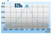
High power LED with 820 lx provides sufficient illumination with only a 174mA current draw.
